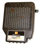
The two FibreIRS 2SATGTU's have been designed to output 8 satellite polarities, DTT, FM and DAB from a single optical input. Two versions available, Quad with 4 universal IF outputs with terrestrial available on each with DiSEqC commands used to switch between the two satellites. Quatro version has 8 fixed polarity IF outputs and a separate terrestrial connector
