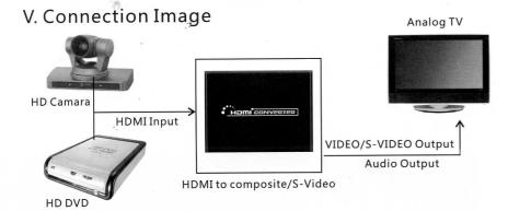
Note: This product doesn't support simultaneous output of Composite Video and S-Video. Please select either one of them by switch button on the unit.
